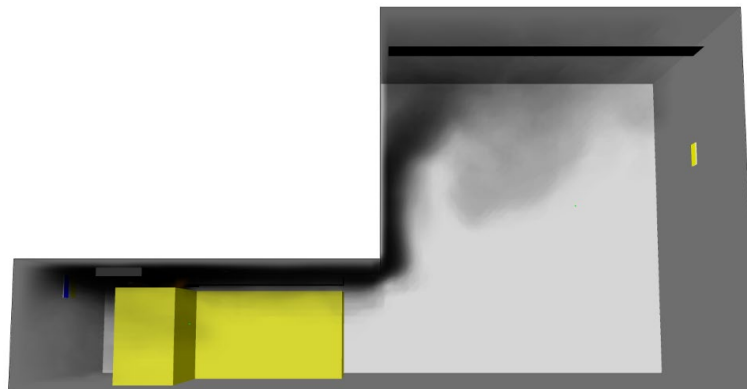
Figure D-9. FDS/Smokeview representation of the MCC/SWGR scenario.
